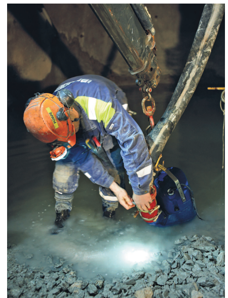
Fig. 3. Sulzer submersible drainage and sludge pumps XJ/XJS for mines
