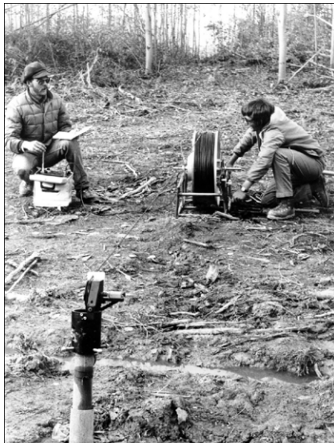
The prototype Borehole Pulse EM system
