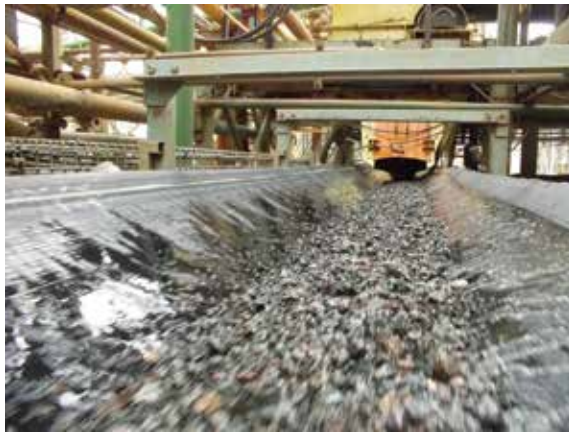
Control of material from the transfer point is critical to optimise belt life
