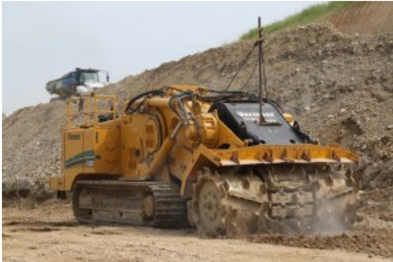
Mark Cooper, Jeff Flahive and Jim Hutchins were the development team for Vermeer to introduce its first Terrain Leveler® surface excavation machine (SEM) in 2002. The company says “the innovative Vermeer® T1255III Terrain Leveler SEM offers superior production in a variety of applications, including surface mining. Depending on the model, a Terrain Leveler SEM can cut areas up to 4.6 m wide and up to 813 mm deep in a single pass.” A patented, industry-
