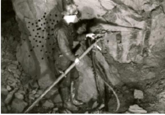
Application of a lightweight Atlas Copco drill with pusher leg in a Swedish mine
